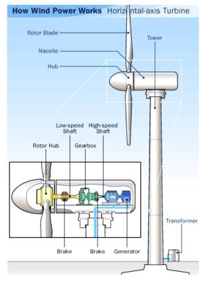
A wind turbine turns wind energy into electricity using the aerodynamic force from the rotor blades, which work like an airplane wing or helicopter rotor blade. When wind flows across the blade, the air pressure on one side of the blade decreases. The difference in air pressure across the two sides of the blade creates both lift and drag. The force of the lift is stronger than the drag and this causes the rotor to spin.
